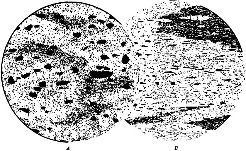
FIG. 93.—CHLORITE-SERICITE-SCHIST (Devonian), Delabole, North Cornwall; \times 60 . Showing sections parallel and perpendicular to the schistosity or cleavage. The main constituents are sericitic mica, chlorite, ilmenite, magnetite, and quartz.
